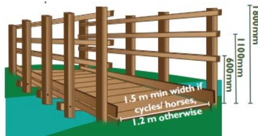
Fig. 3b – Typical bridleway bridge design
