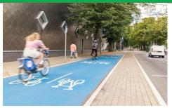
A physical feature, such as a kerb or a change in surface material, separates cyclist and pedestrian spaces, or a separated cycle route runs alongside a road, distinguished by vertical barriers, coloured asphalt/paint, or elevation differences.
