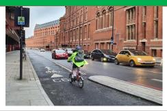
Infrastructure that allows people cycling to ride in the opposite direction to one-way motor traffic. It is best implemented by raising the route to footway level or via a protected lane at the road level.
