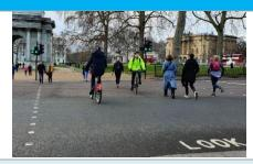
An unsegregated signal-controlled crossing for pedestrians and cyclists, linking cycle track and footway systems on opposite sides of a carriageway.
