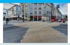
An all-red traffic signal phase that allows green time for pedestrians to cross at busy junctions in every direction, including diagonally, at the same time.
